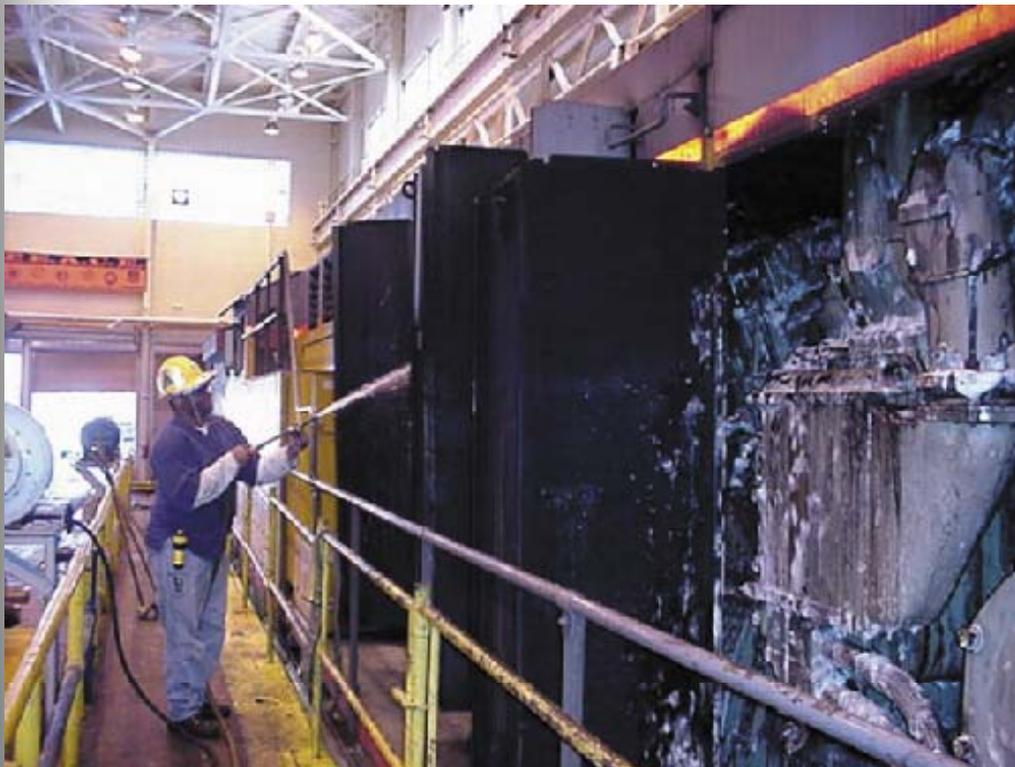
**Engine cleaning process:** operator is applying foam in the background. CleanSafe has already been applied to the engine in the foreground and is self-cleaning the engine.
