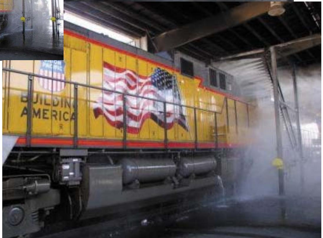
The Locomotives go through the high-capacity washing facility in under 5 minutes.
