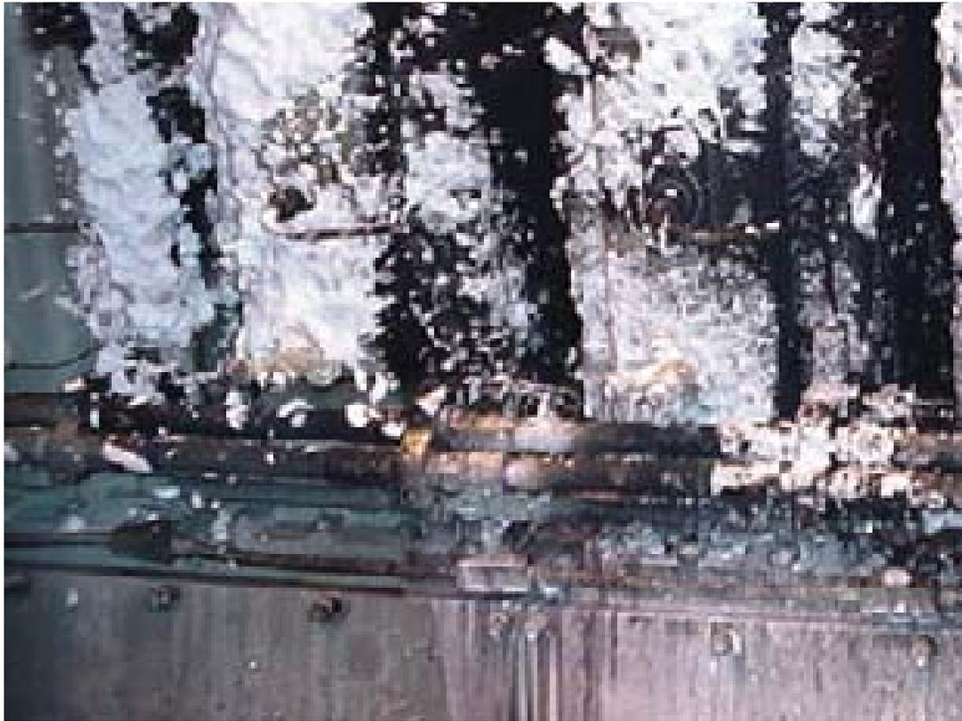
Apply LOCOCLEAN on engine with low pressure sprayer
